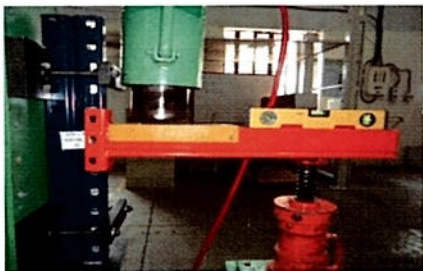
Shear capacity test on Beam end connector - Godrej.
